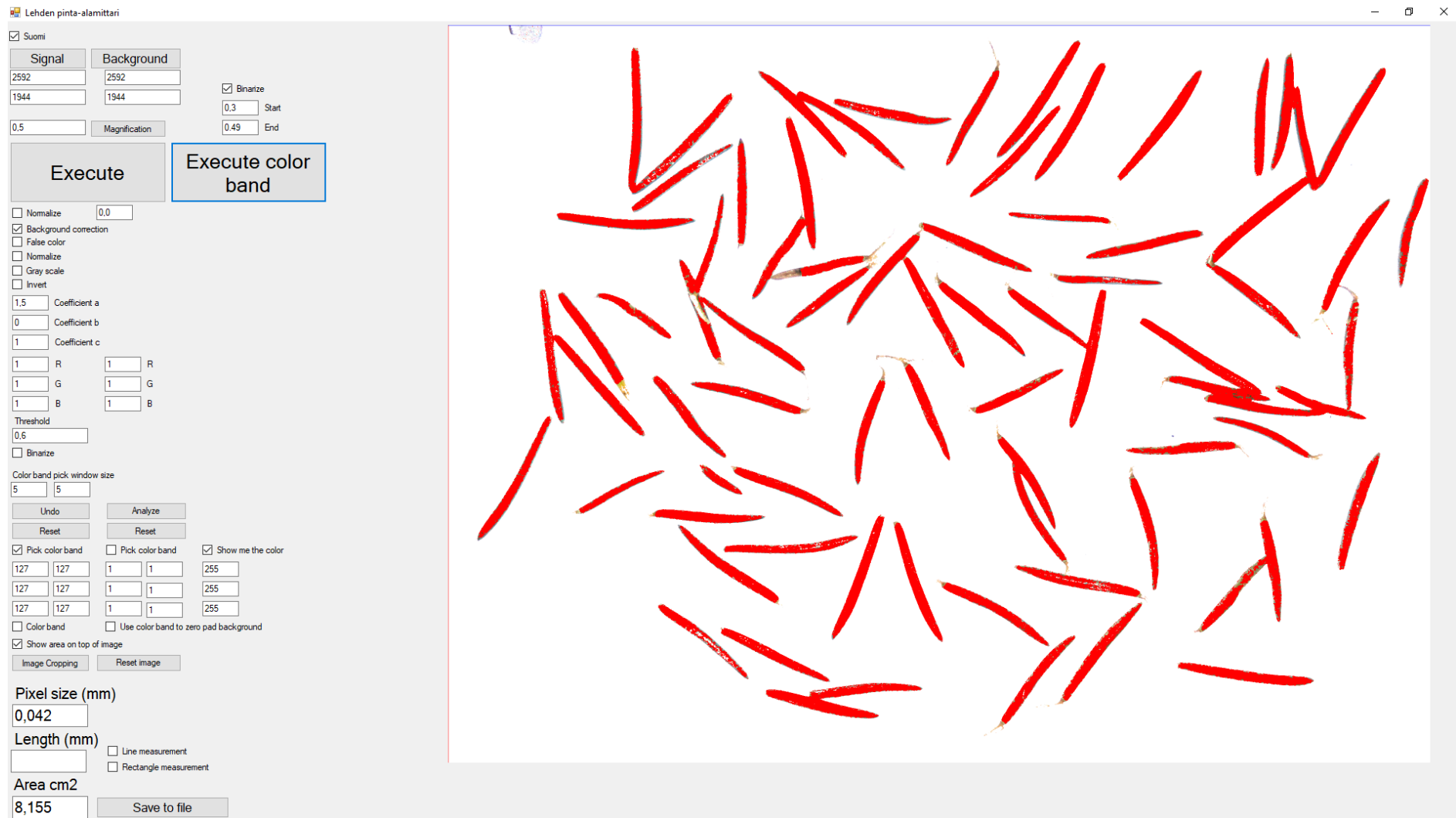
Fig. 9b. Needles separated from the trunk of a spruce branch, which is shown in Fig. 8a. Needle area is 8.155 \text{ cm}^2 , which indicates that magnitude of shading effect is (8.155 - 7.515 \text{ cm}^2) / 8.155 \text{ cm}^2 \times 100\% \sim 7.8\% .
