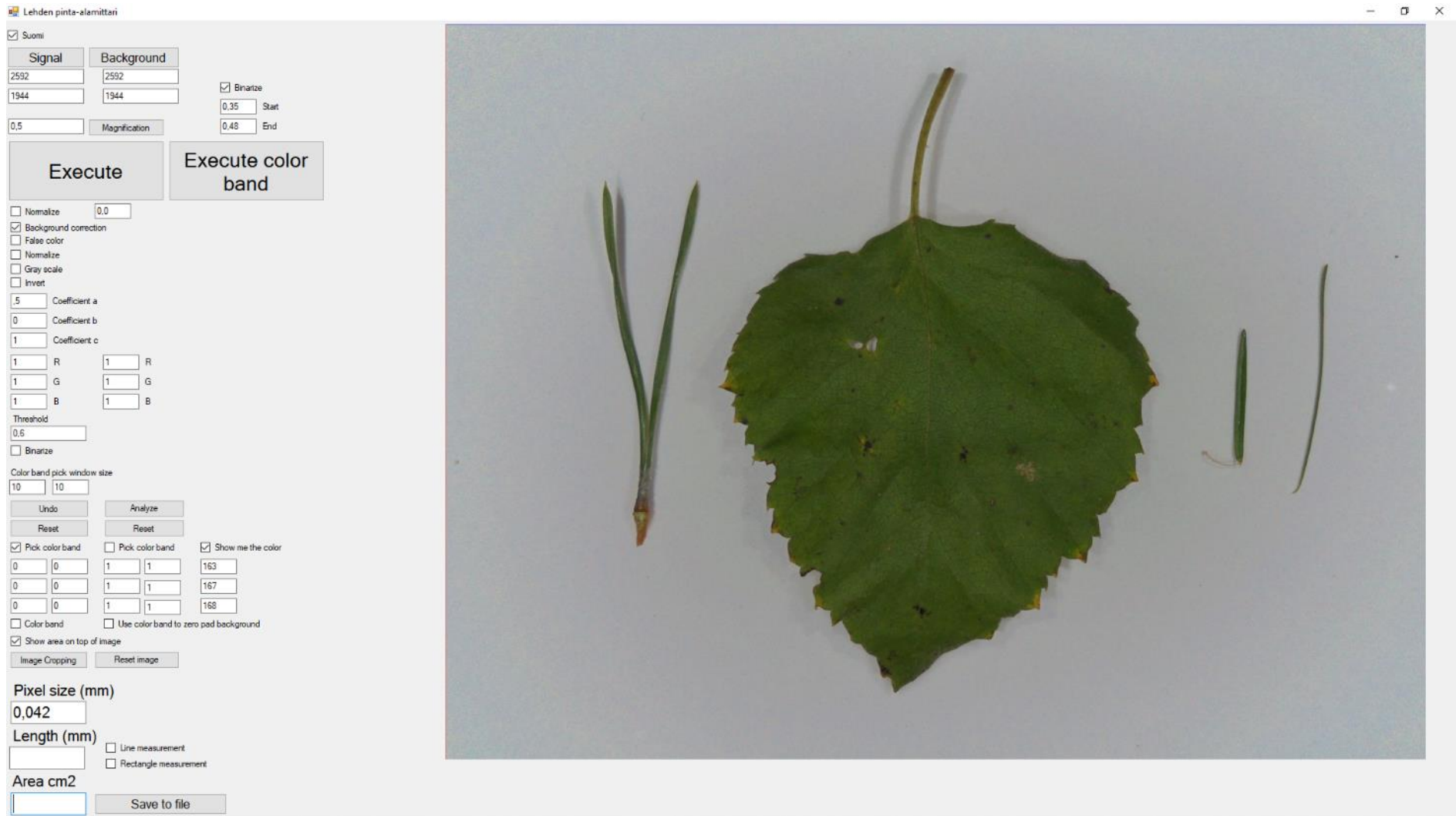
Fig. 5. LePaM -v1 computer program icon. Utilizing this it is possible to measure distances and calculate leaf areas.
