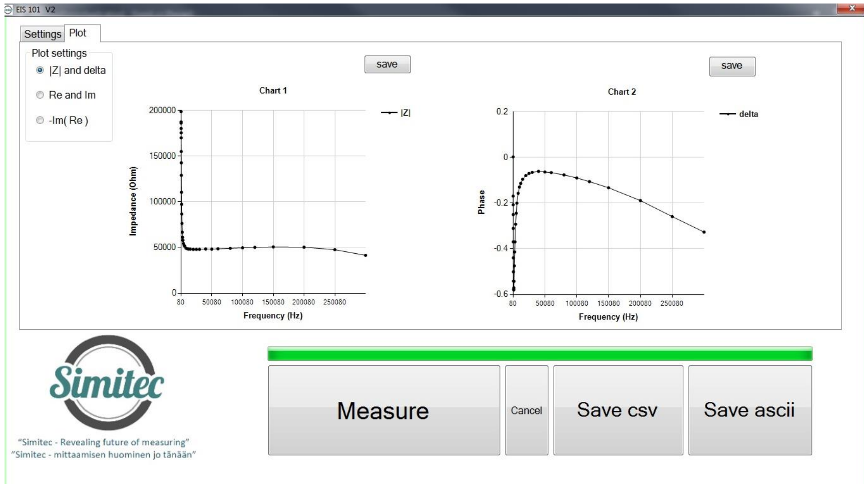
Fig. 5. EIS-101 v2 plotting domain, where the scan of the measurement results ("Plot") within the program is activated. It is also possible to record data from this icon using "Save csv" and / or "Save ascii". Additionally, saving images to jpg format can be done using the "save" keys.
