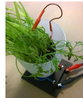
Fig.5. Seedling cell for EIS measurements.
