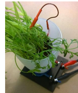
Fig.5. Seedling cell for EIS measurements.
