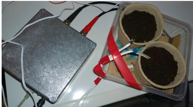
Fig. 4. EIS electrodes in soil for freezing test and the effect of severity of freezing to |Z| responses.
