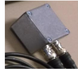
Fig. 2. Calibration impedance cell.
